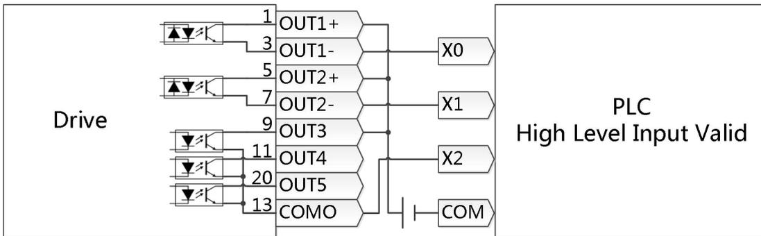
Figure 3-5: Digital output, NPN wiring
