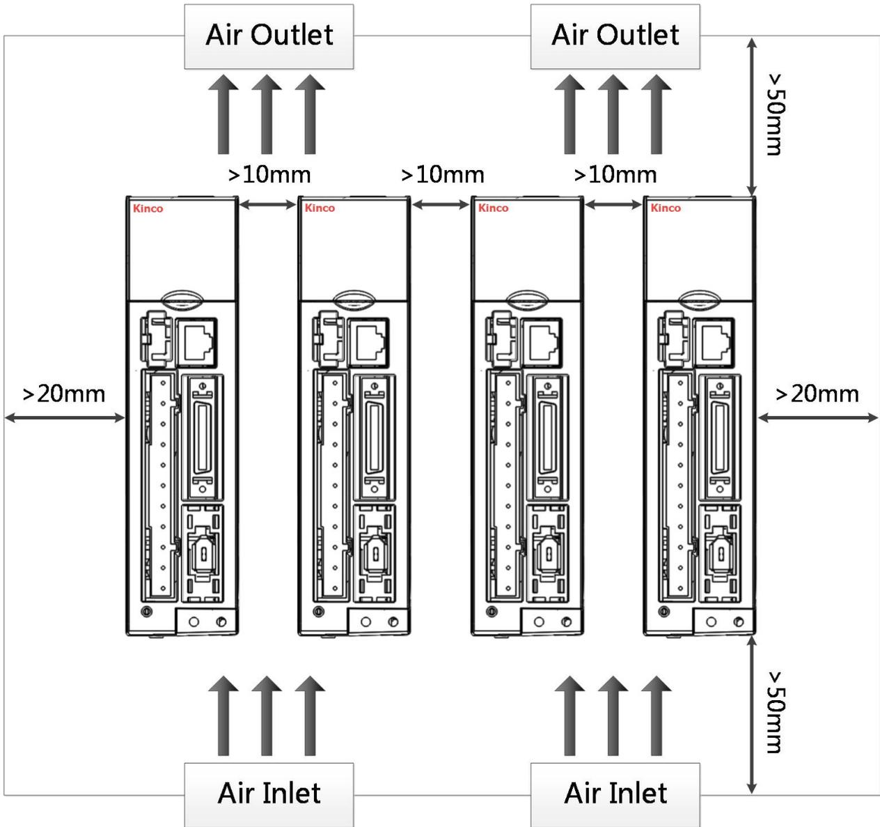
Figure 3-1: Installation orientation, distances and clearances
