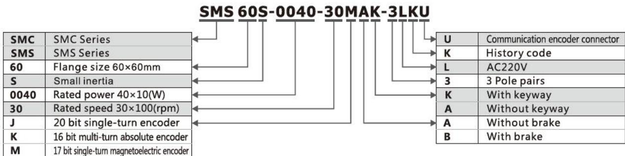
Figure 2-2: Servo motor type code
