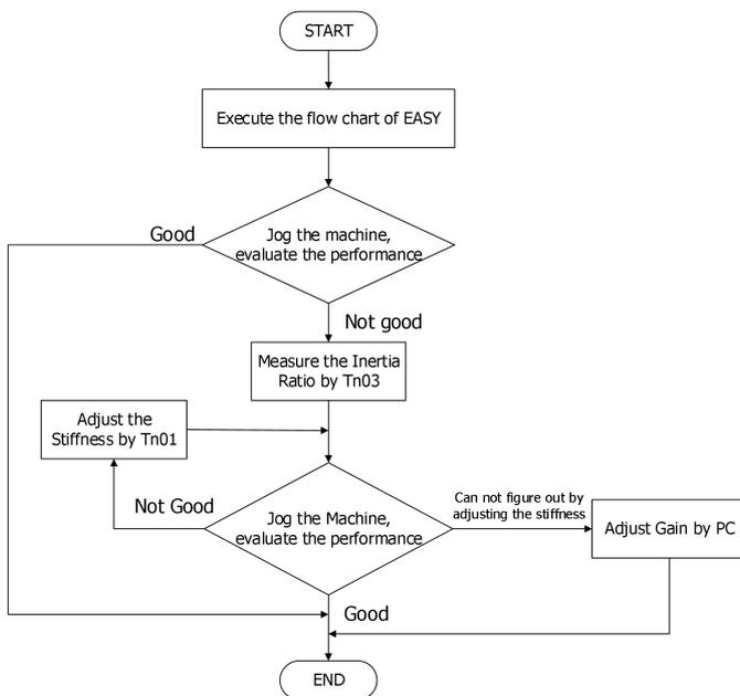
Figure 4-2: Flow chart of the Easy Use function
