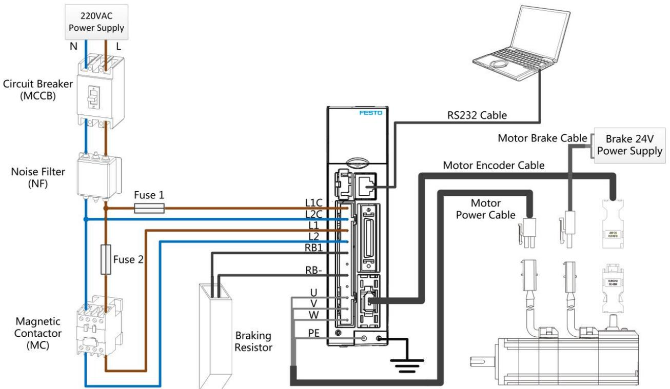
Figure 3-7: Wiring of the CD3 servo system
