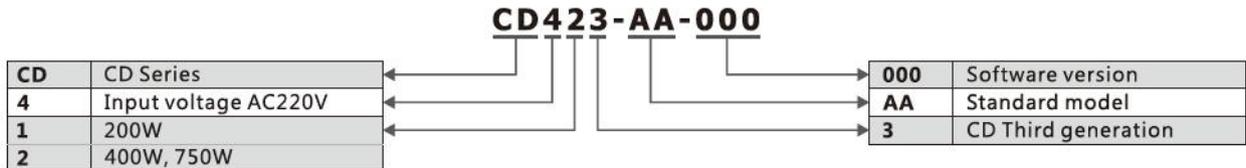
Figure 2-1: motor controller Type code
