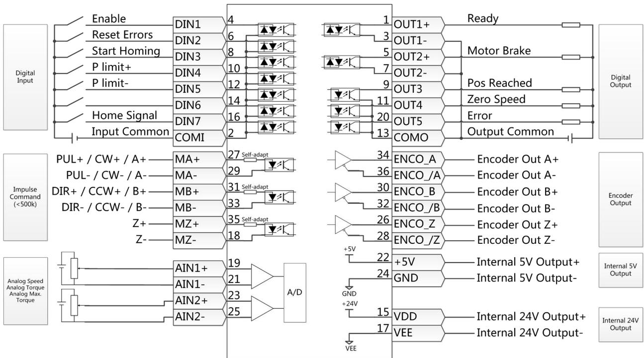
Figure 3-4: X4 wiring
